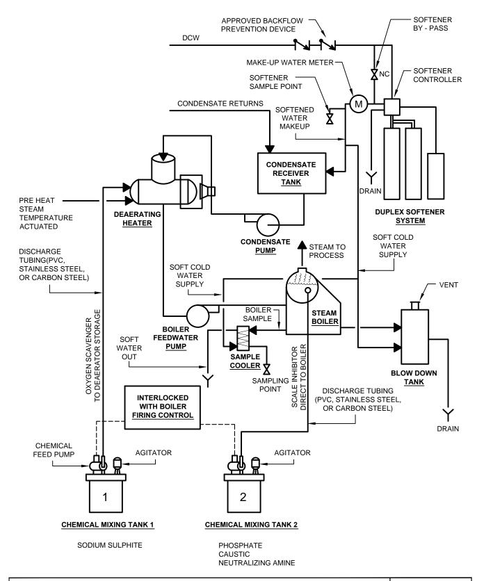
Installation of Chemical Metering System for Steam Boilers
