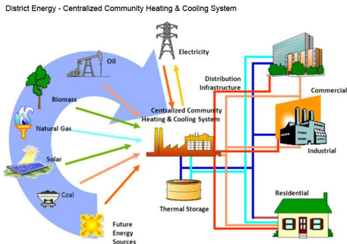
Figure 2 – Schematic showing typical district energy system – Possible heat sources are shown on the left; possible applications on the right. Photo credit – Google Images
