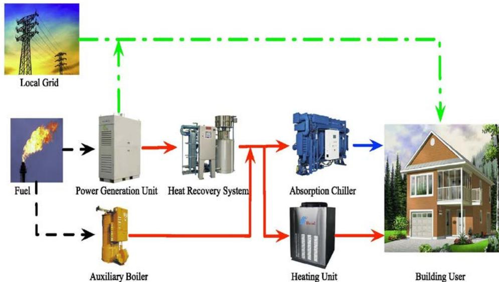
Figure 4 – Schematic showing typical parts of a CCHP system – Photo credit – (Liu et al., 2014, p. 2)
