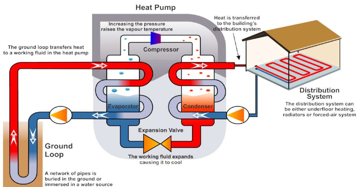
Figure 14 – Schematic of a Geothermal Heat Pump - Photo credit – Google.
