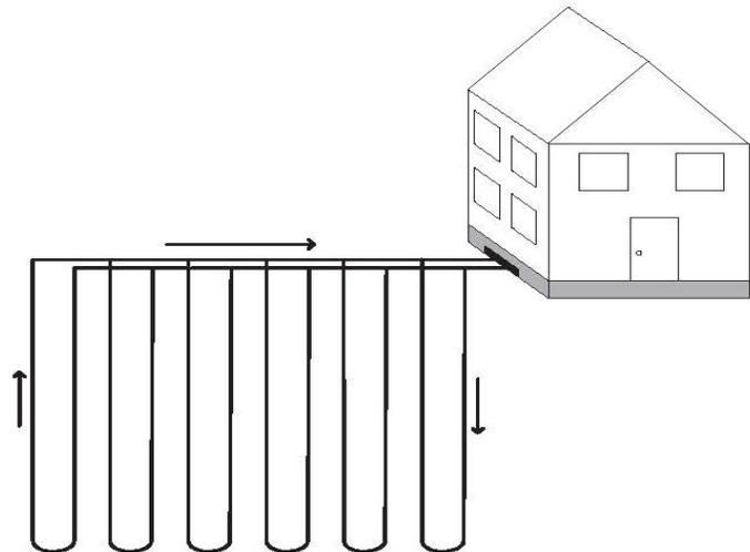
*Figure 8 – Vertical closed loop heat exchanger for a geothermal heat pump - Photo credit – Self et al., 2013.*
